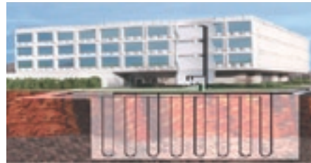
The vertical closed loop geothermal system used by KeyMed (artist’s rendition). The loop absorbs energy (winter) and discharges energy (summer) to provide heating and cooling.
