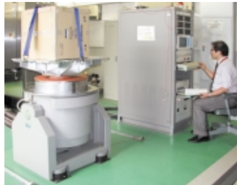
Vibration Test of Packaging
