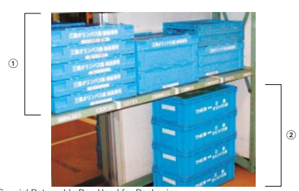
Special Returnable Box Used for Packaging ① Folding plastic box. The shock absorbent-material inside is returnable. ② Plastic cardboard. The shock-absorbent material is for exclusive use.
