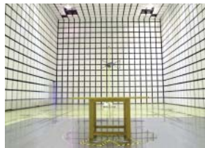
10-m radio wave anechoic chamber in the Test and Evaluation Center
