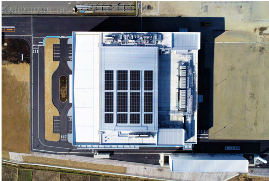
Solar panels installed on the roof can be seen in the center of the photograph (total generating capacity of 180 kW)
