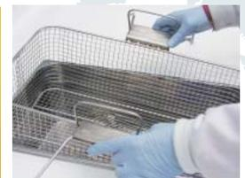
Cleaning process of HF electrodes before sterilization.
