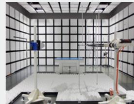
Electromagnetic field immunity test chamber
