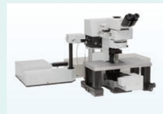
FLUOVIEW FV1200MPE multi photon laser scanning microscope
