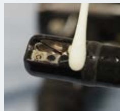
Sampling from endoscope distal end
