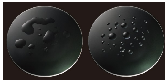
Oil-repellent coating with (right) / without (left)
