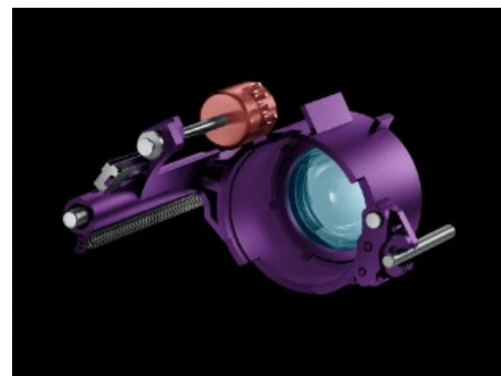
MSC (Movie and Still Compatible) mechanism
