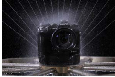
Image of splashproof testing
