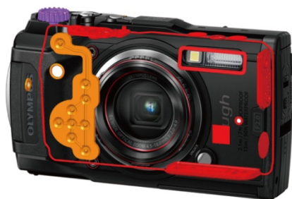
Image of Sealing Construction
