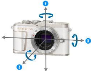
Image of in-body image stabilization
